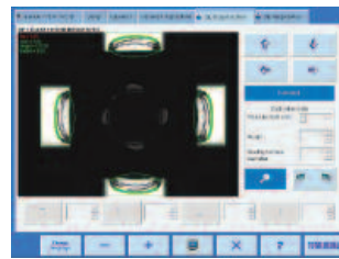
Vision dip/saddle inspection image showing four overlapping side views of the container finish
