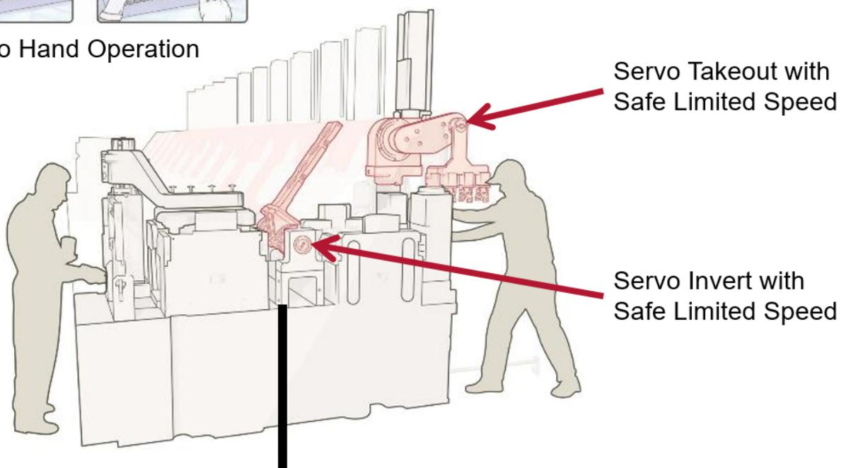
Safe Separation of Blank and Blow Side Operation
