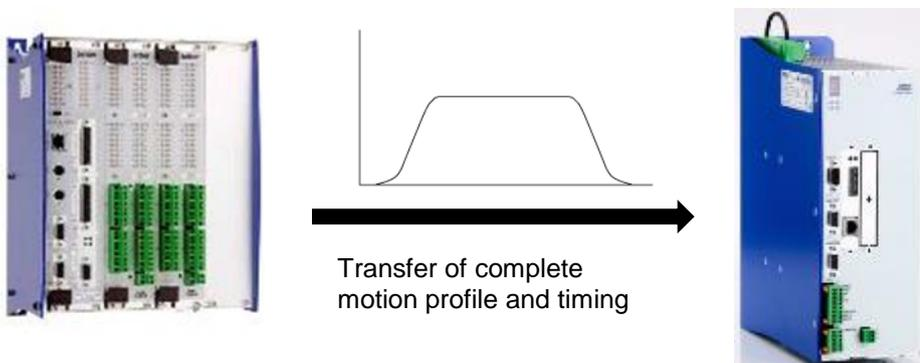
With **FlexIS 3** the controller uses the Motion Control technology and transfers the set point every 2-4 ms.
