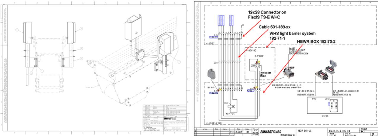
The WHS System is completely integrated in the TS-E WHC configuration.
