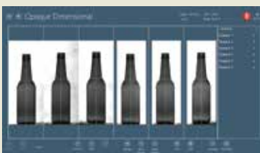
Flex BC - C-side Dimensional Dimensional measurements calculated from 6 views
