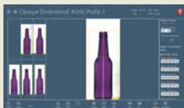
Flex BC - C-side Masking Automatic profile for inspection regions
