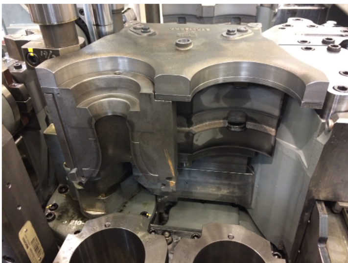
New plenum chamber design allowing individual mold cooling cavity control
