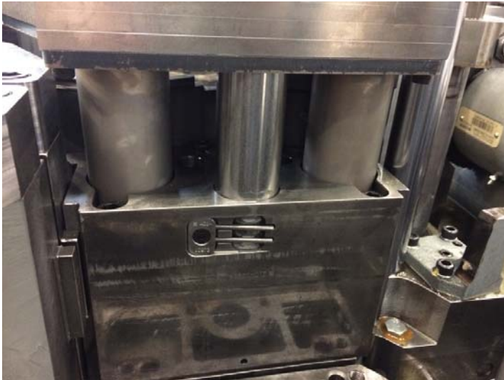
Improved height adjustment of the plenum chamber
