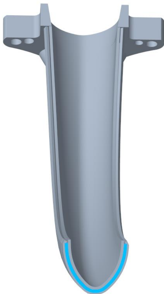
Bezier type cooling chamber
