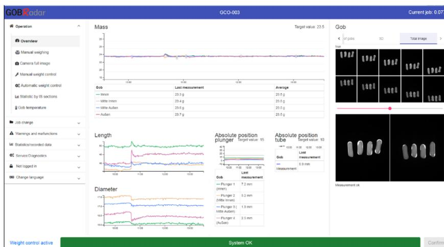
**Compare gob form Screen** - The shape of the gobs can be stored for reference and compared to current production. This is especially helpful during job change to reproduce the “last time best shape” but also for continuous monitoring during production.
