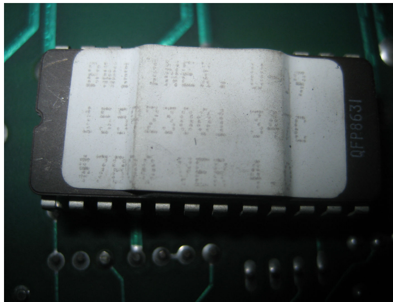
Figure 2: Close-up of EPROM showing software part number and version. In this case, the software part number is 155923001.
